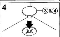
Attach Housing Cap(3) & (4) to each Klix Cam(2) by pushing the neck thought the center of the Klix Cam,
