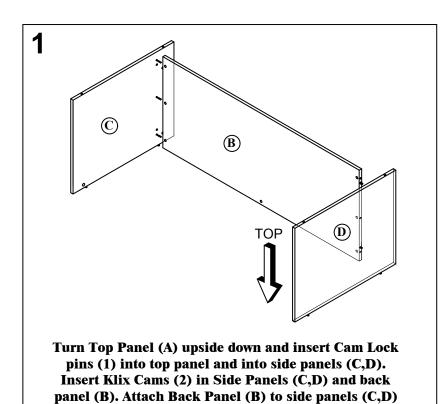
and Top Panel (A). Turn Klix Cam to tighten.
